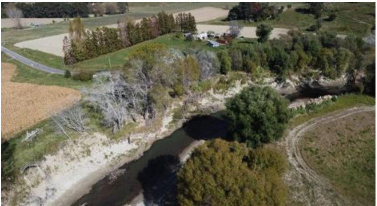
Figure 28. Densely treed outer bends suffered little bank erosion, but silver poplars (foreground, left bank) were undermined by toe erosion.
