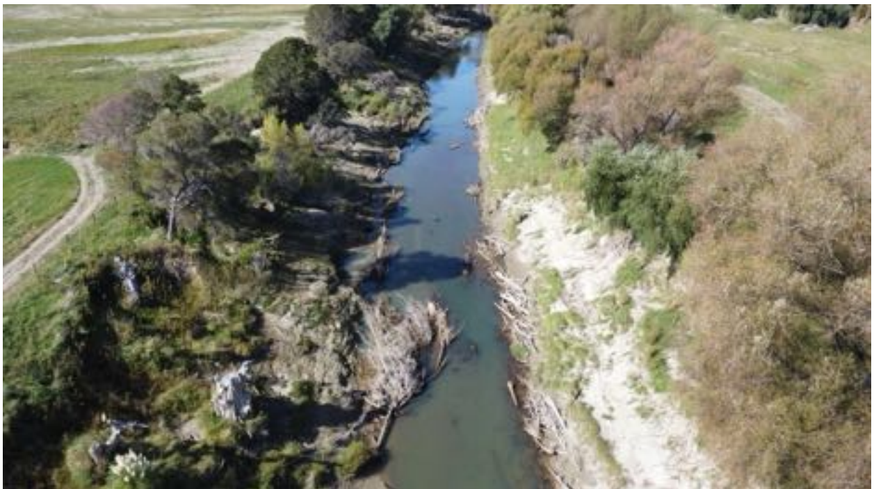
Figure 26. Bank stabilisation by tree willows (right bank) contrasted with slumping into the channel on left bank (despite the presence of mature mānuka and other tree species).
