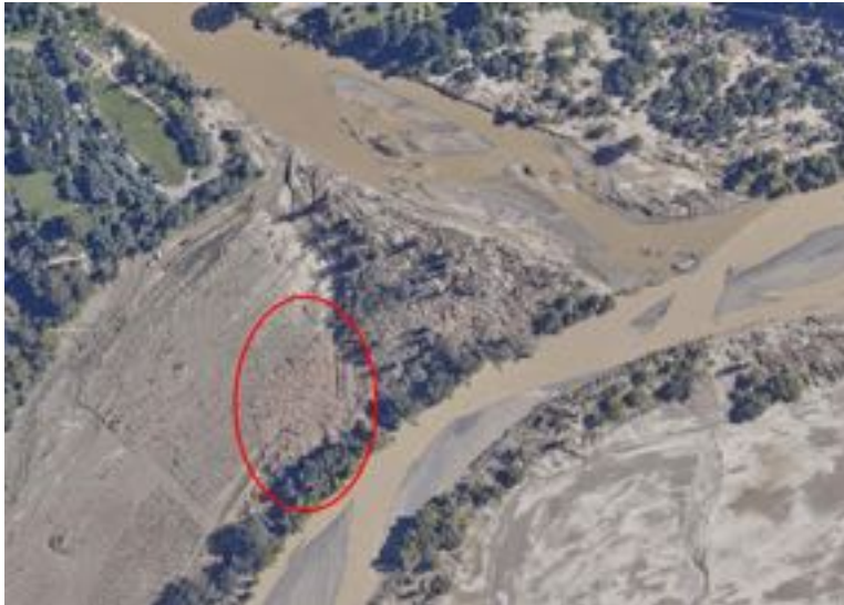
Figure A34. Floodplain woody debris capture— Tūtaekurī & Mangaone River confluence.
