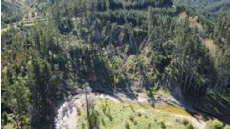
Figure A24. Major slip carrying mature pine trees into the river bed – Hikuwai catchment.
