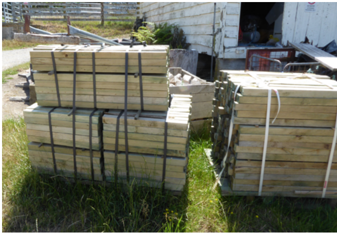
Figure 3. Left. Poplar battens bundled on a pallet on farm for delivery to the treatment plant.
