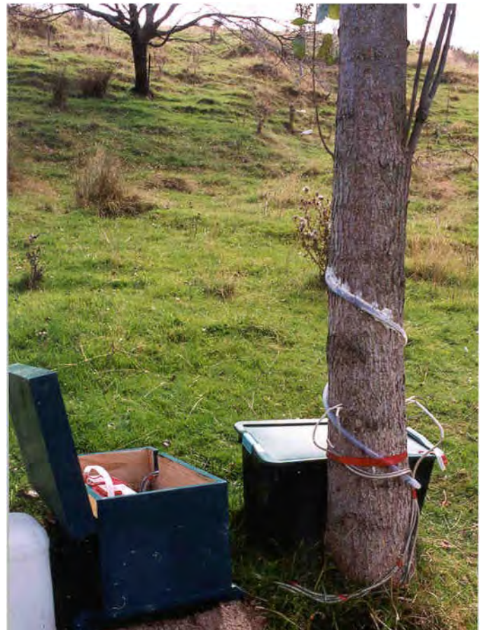
Stem flow captured in a plastic gutter and stored in a 40L container
